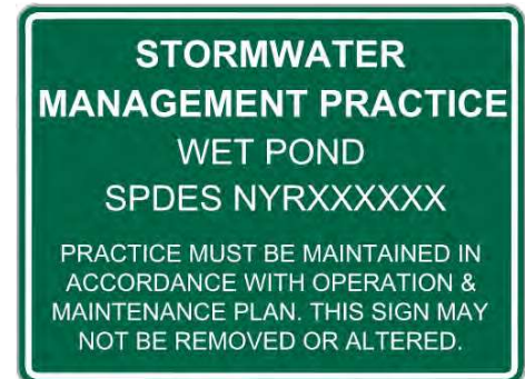
Figure 3.1 Example Post-Construction Stormwater Management Practice Sign
