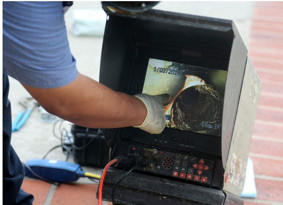
Above: An inspector looks inside the sewer with a special remote-controlled camera.
