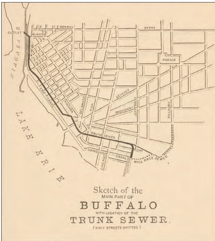
The Trunk Sewer, indicated by the heavy black line, was primarily constructed to flush the Hamburg Canal and Wilkeson Slip, and only incidentally carried sewage to the Niagara River from inland sewers.
