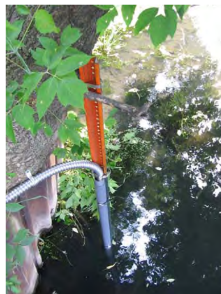
Level sensor stilling well at North bank (just upstream of dam)
