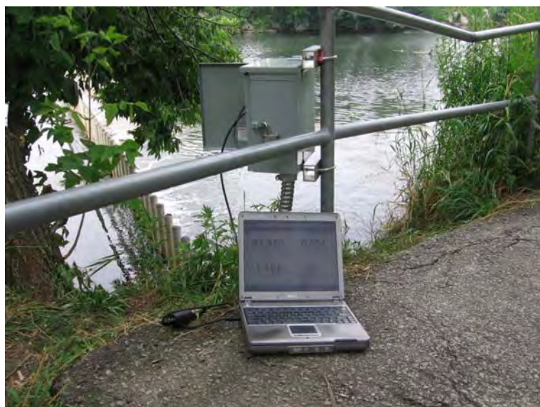
Level sensor download box on North bank at Grant Street Dam
