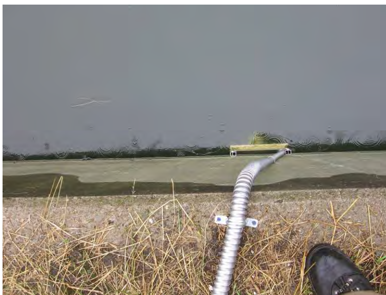
Downstream HADCP mounted on concrete wall
