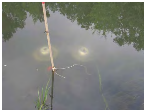
Duplicate in-situ SOD chambers during upstream survey
