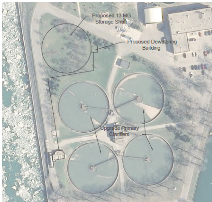
Figure 5-16: Process Flow Diagram for Alternative B4
