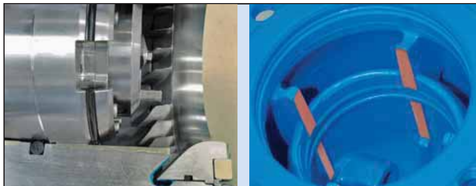
The four surface-hardened guides ensure uniform movement of the piston and contribute to long life.
