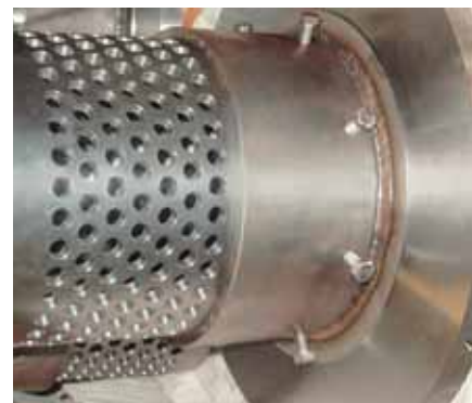
Inline fixed throttling cylinder can be installed at a distance of roughly three times the nominal size downstream of the Plunger Valve when further pressure reduction is required.
