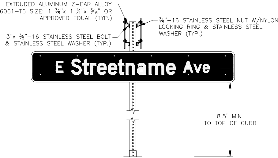
GROUND MOUNT STREET NAME INSTALLATION IF BOTH L ARE \leq 42"
